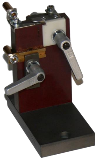
57D01130: measuring device brush body to cable adjustable / for small brushes
